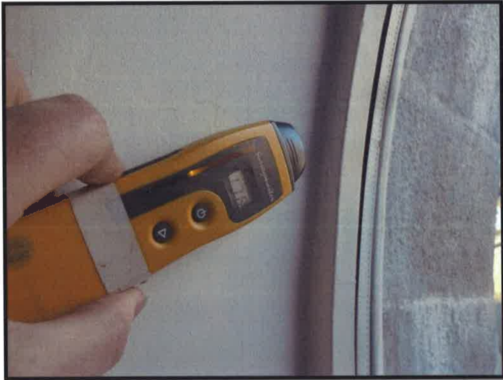
Figure 4 Meter reading (18% as before), repainted surface left hand side (LHS) lounge window
