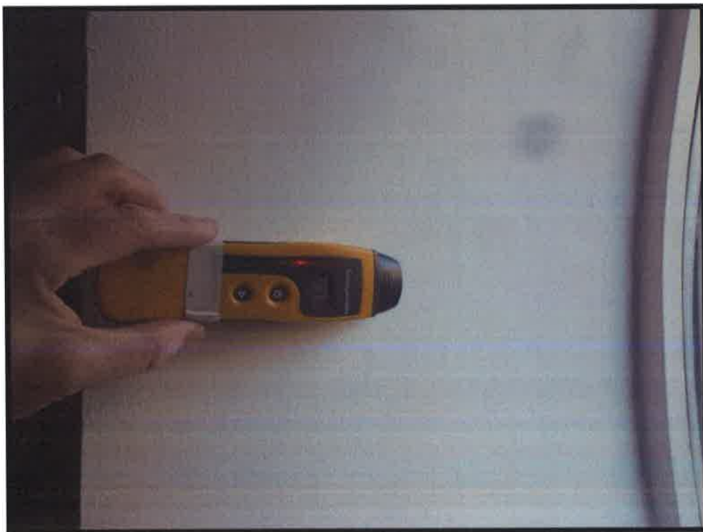
Figure 5 Further meter reading (24%) LHS lounge window, mid level.
