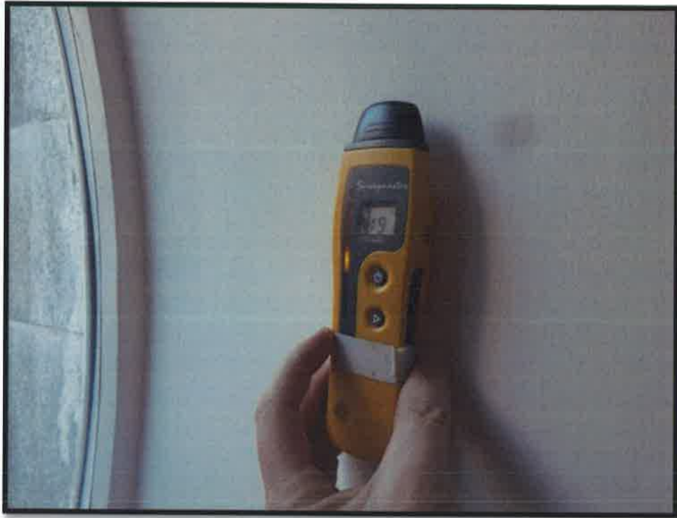
Figure 6 Meter reading (19%) RHS lounge window, mid level.
