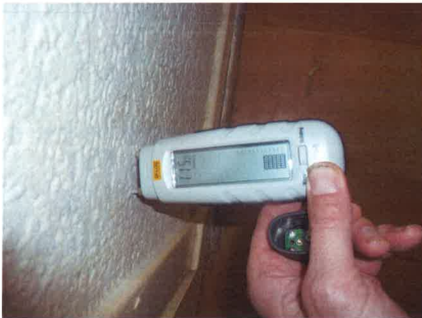
4. Moisture reading – external wall in bedroom.
