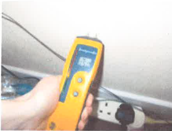
Bedroom - Damp meter readings - amber at base of rear external and party walls
