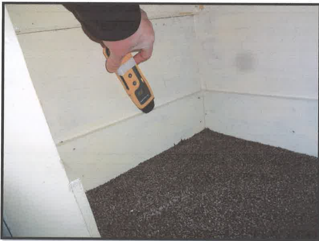
Figure 11 Lounge - Meter reading (18%) inside alcove cupboard at outer wall surface, above skirting
