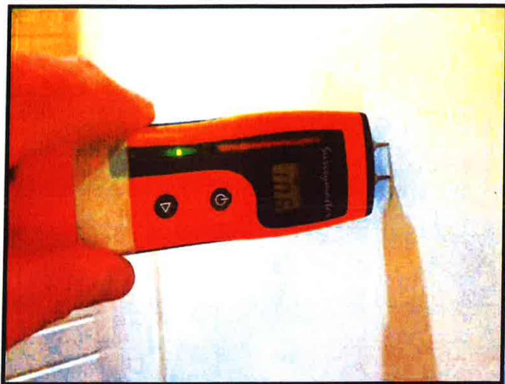
Figure 6 Damp meter reading left side lounge window
