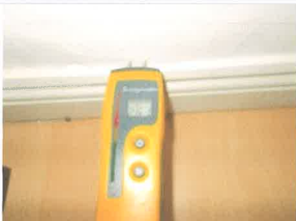
Living Room - high moisture reading to base of external wall
