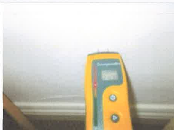
Large bedroom - high moisture reading to base of external wall
