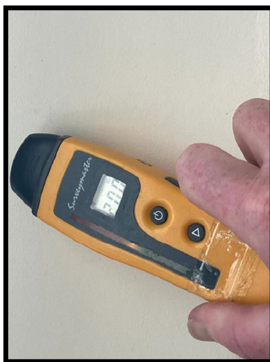
Photograph 13 Kitchen window frame: Moisture reading 20%.
