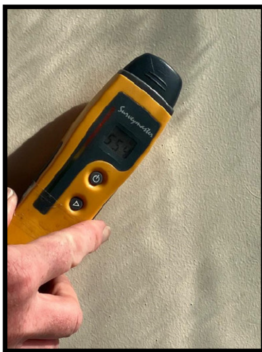
Photograph 14 Kitchen window ingo: Moisture reading 55%.
