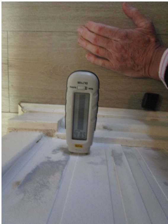
2. Dampness meter reading skirting level hall wall adjacent bathroom door
