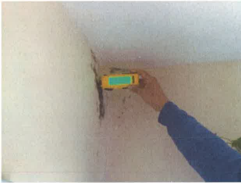
Bedroom 2 – north – damp staining in north west corner
