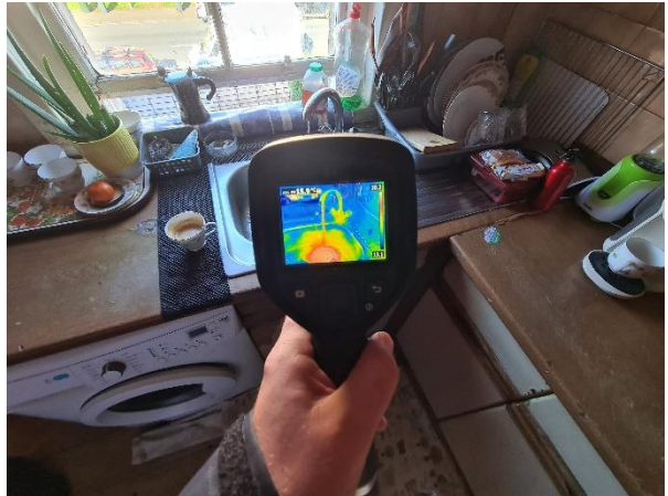
14 Hot water to kitchen sink.
