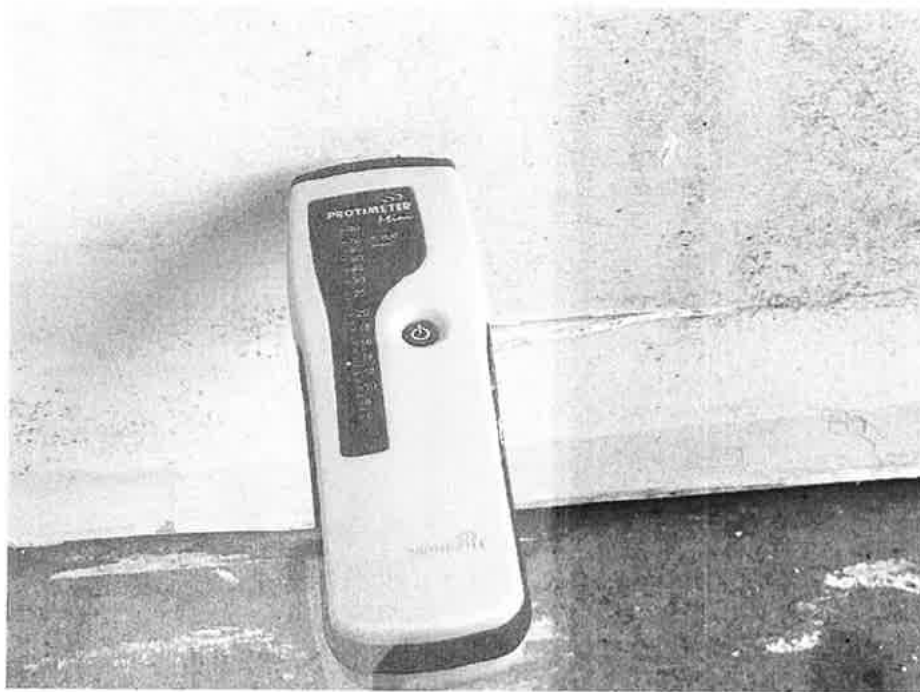
12 – “Protimeter” reading in utility area
