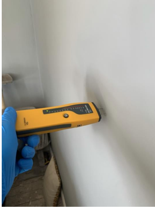
Photograph 6: Living room wall (damp meter shows moisture levels not excessive)
