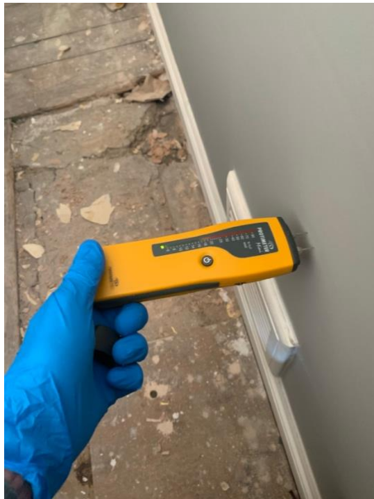
Photograph 5: Living room wall (damp meter shows moisture levels not excessive)
