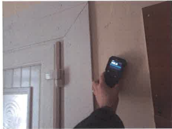
27 High moisture readings within Kitchen.
