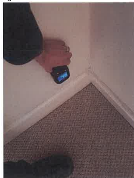
23 High moisture readings within Dining Room.
