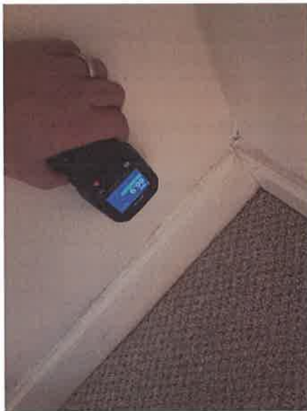
24 High moisture readings within Dining Room.
