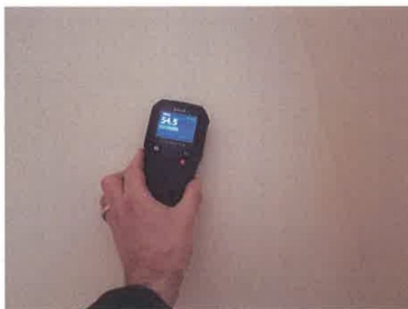
22 High moisture readings within Dining Room.
