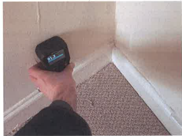
25 High moisture readings within Dining Room.
