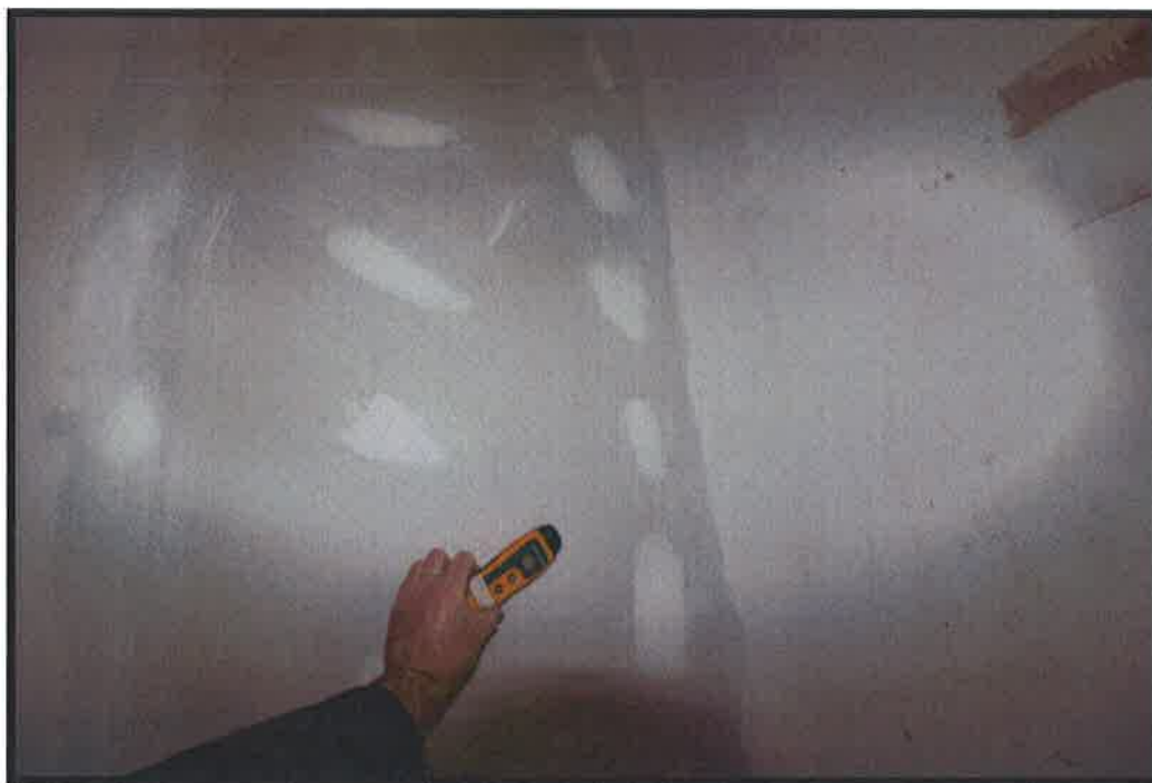
Figure 4 Front Bedroom typical moisture meter reading (12%) (previously 15%)
