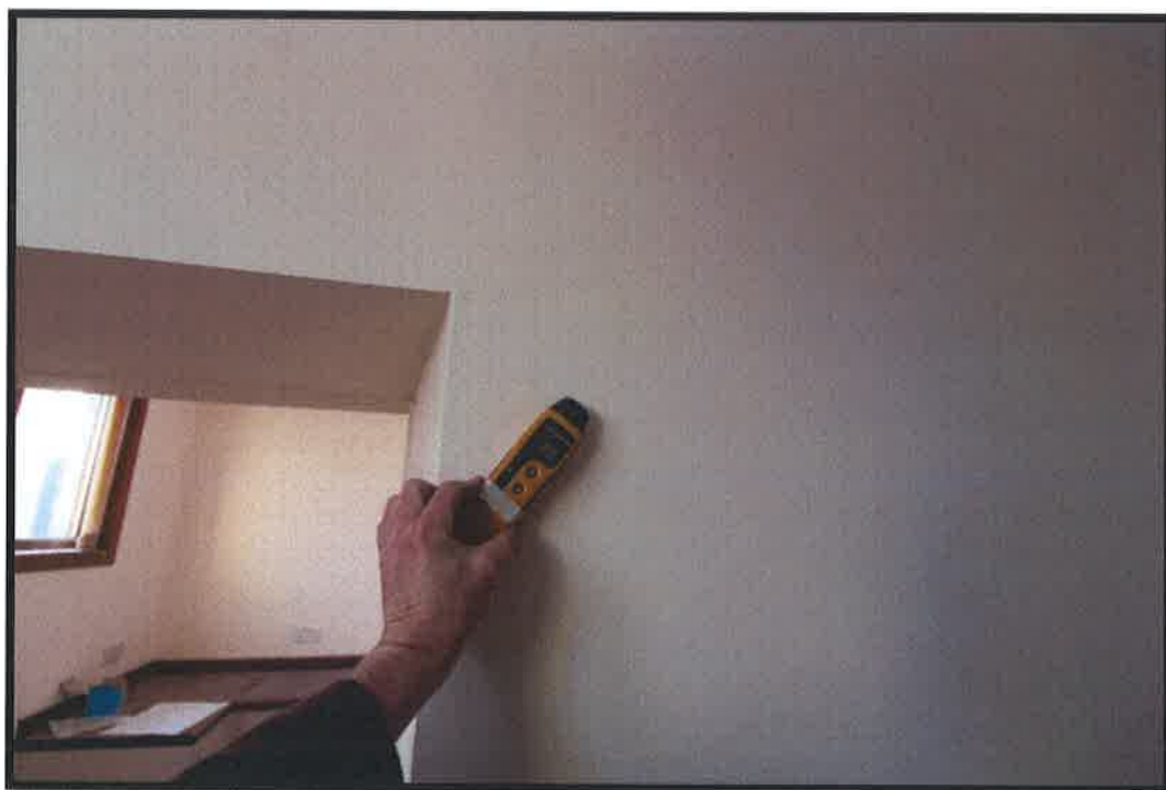
Figure 11 Doorway to utility room(new kitchen) - Meter reading (9%)(previously 100%).
