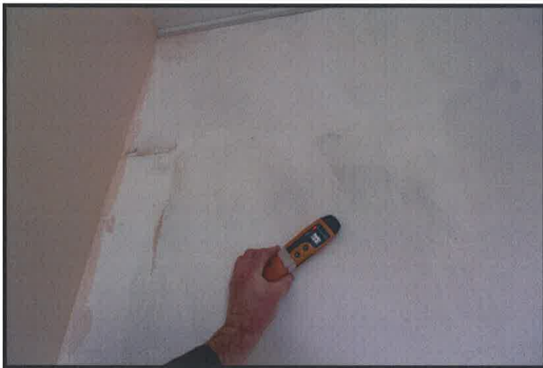
Figure 12 Kitchen - side wall adjoining bathroom, high level. Moisture meter reading (100%)
