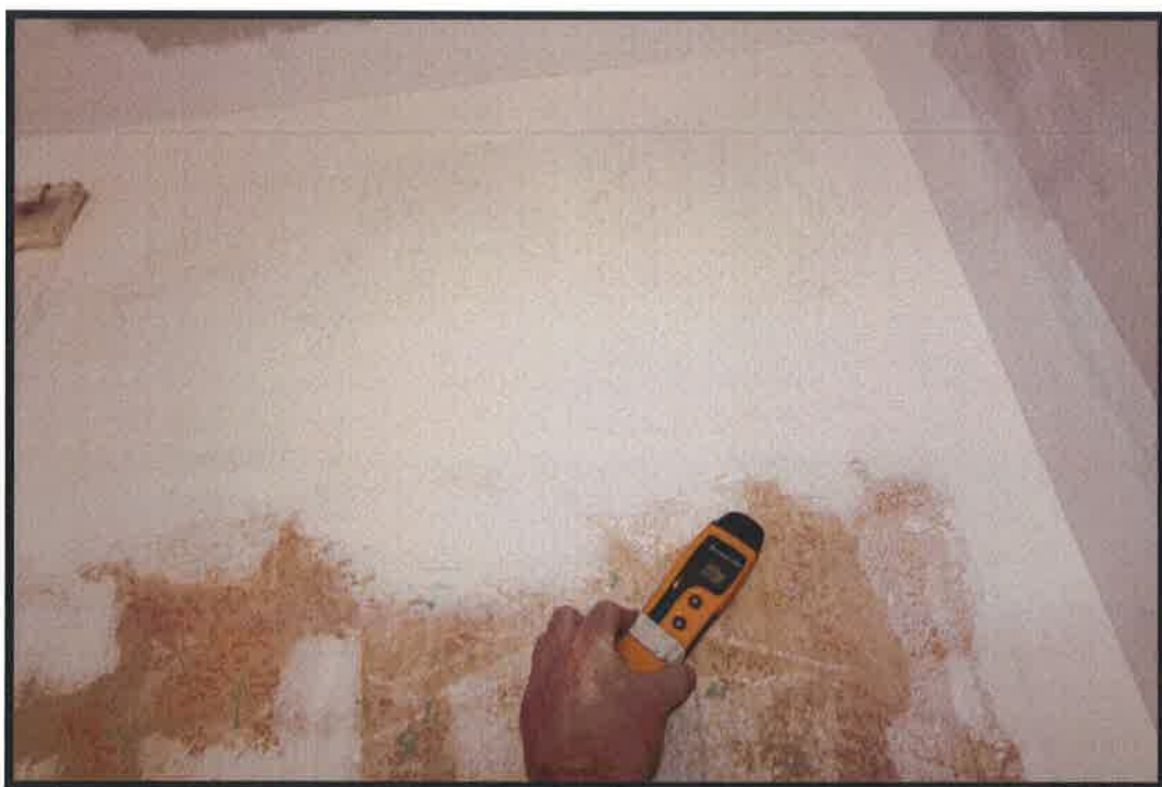
Figure 9 Rear bedroom - Meter reading (16%) rear corner at outer wall (as before).
