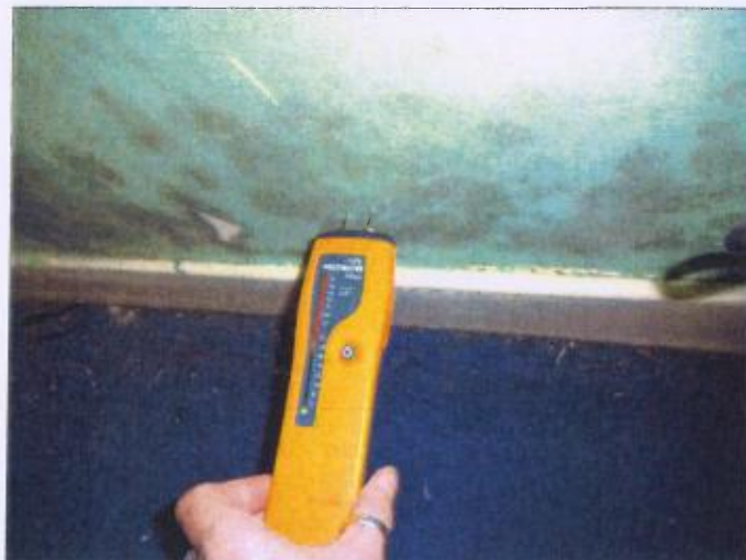
No evidence of dampness in bedrooms - Mould due to condensation
