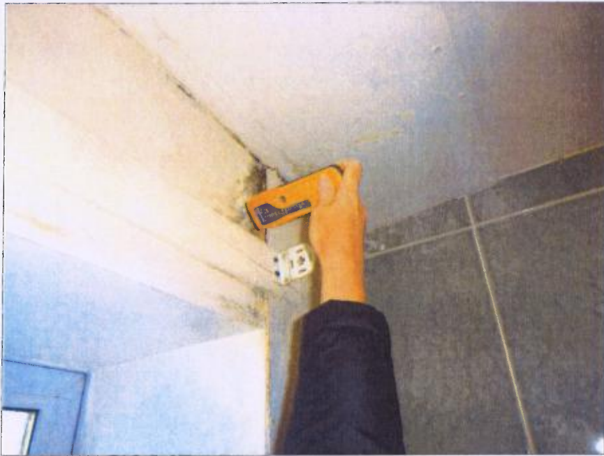
No evidence of dampness in bathroom – Green moisture meter readings recorded Historic water staining noted
