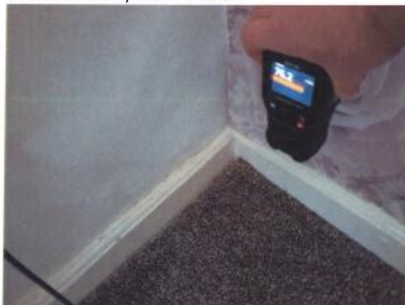
17 High moisture meter readings recorded at low level within Front Bedroom wall.
