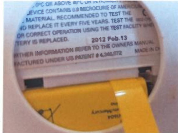
2 Removable battery to smoke detector and date stamp.
