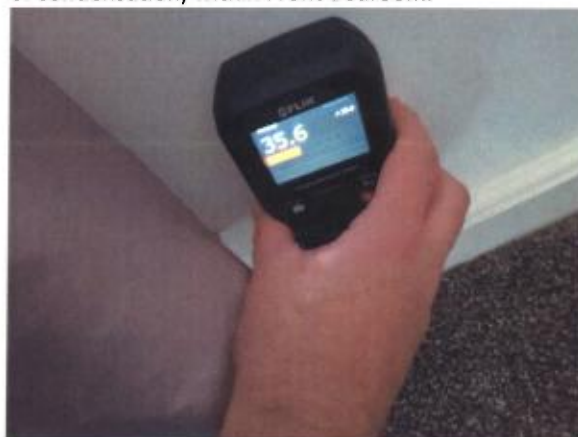
18 Further example of high moisture meter readings recorded at low level within Front Bedroom.
