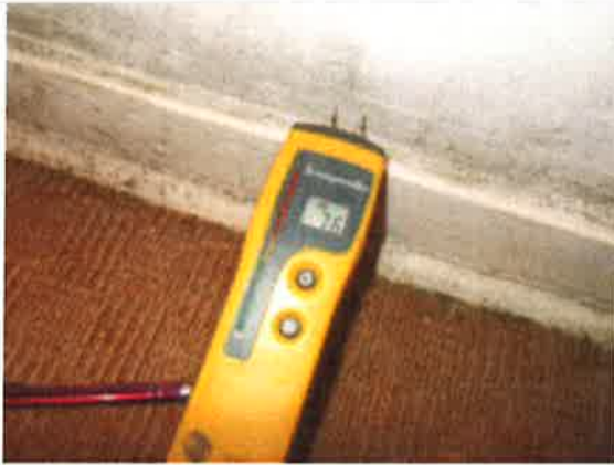
Bedroom - low moisture reading to base of wall adjacent to wardrobe
