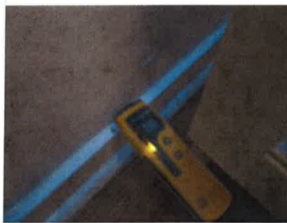
Bedroom - moderate moisture reading to base of external wall below window
