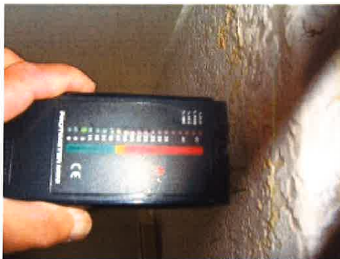
“Green” reading on moisture meter at LR chimneyhead
