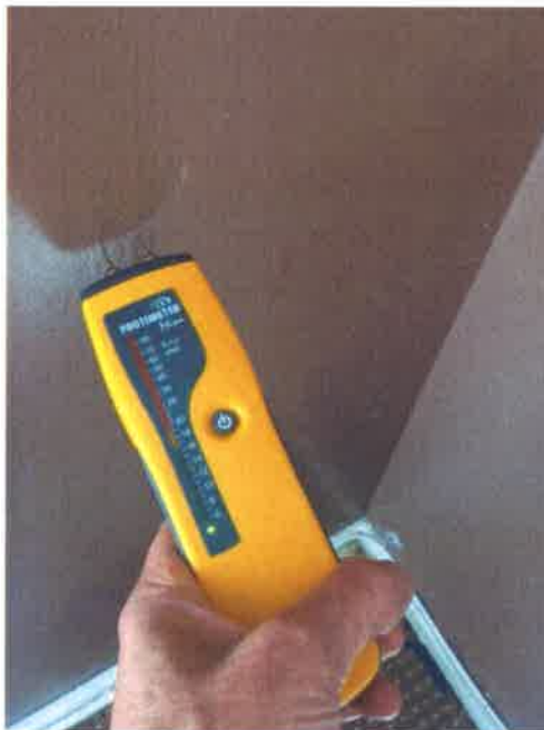
Photograph 10: Living room: wall - damp meter reading – interior
