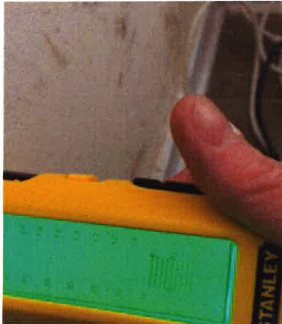
DAMP METER READING TAKEN BELOW LIVING ROOM WINDOW
