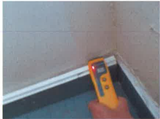
Living Room - high moisture reading to base of gable wall.
