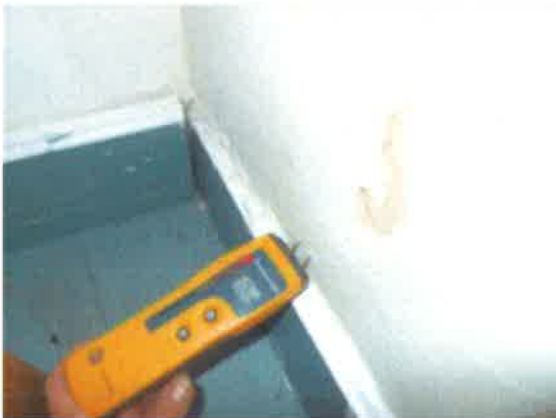
Living Room - high moisture reading to base of party wall to back bedroom
