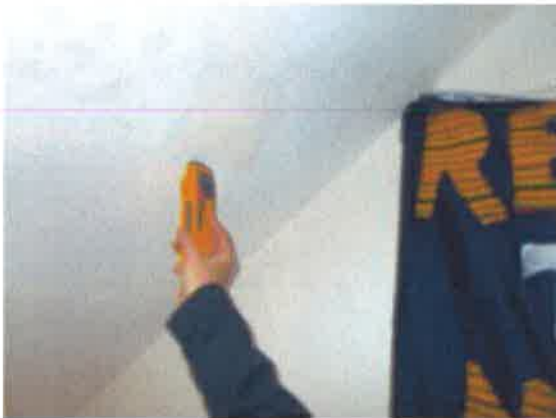
Living Room - high moisture reading at damp patch on camceil ceiling on right side of dormer window
