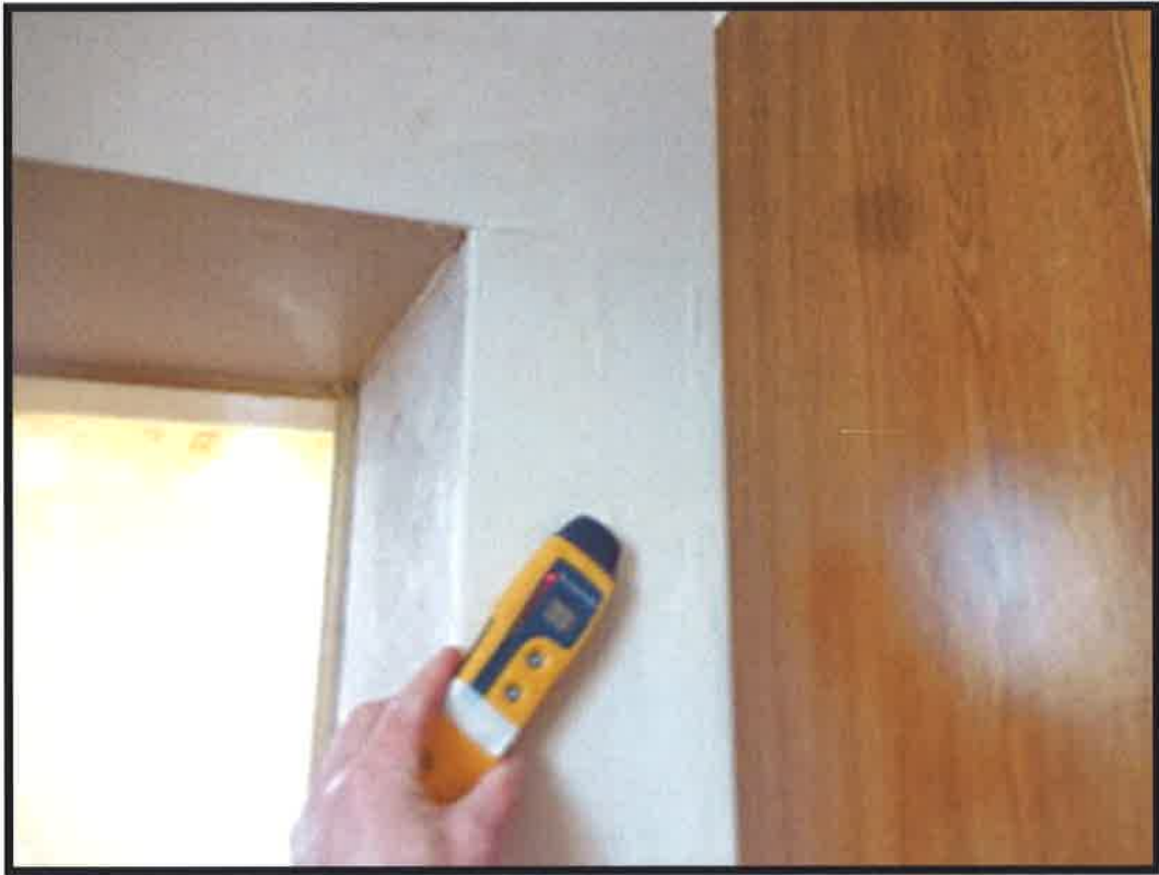
Figure 115 Doorway to utility room - Meter reading (100%).
