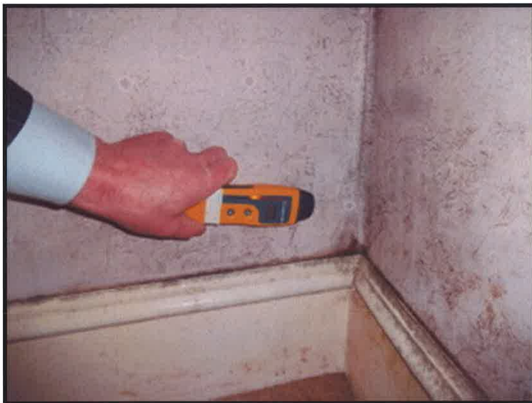
Figure 11 Rear bedroom - Meter reading (19%) rear corner at outer wall.
