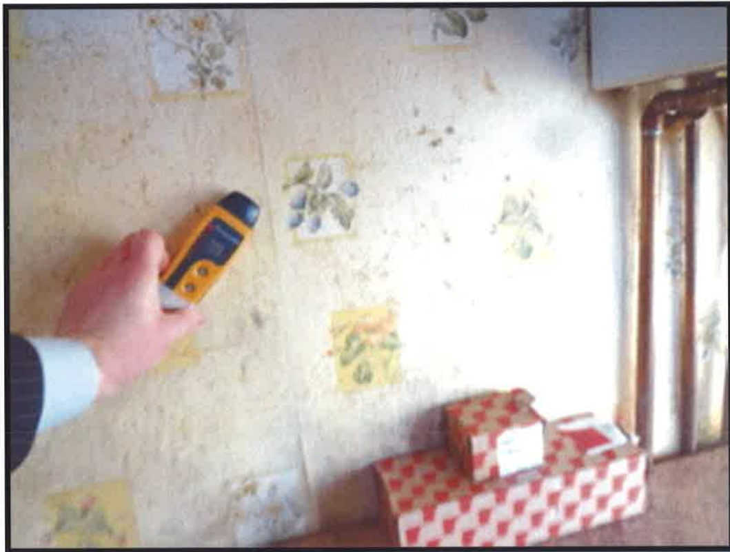
Figure 148 Utility room - moisture meter reading (100%)
