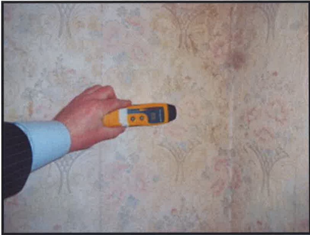
Figure 4 Front Bedroom typical moisture meter reading (15%)
