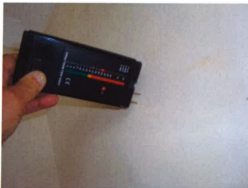
STAINING AND HIGH DAMP READINGS AT FRONT BEDROOM CHIMNEYBREAST (12/04/17)
