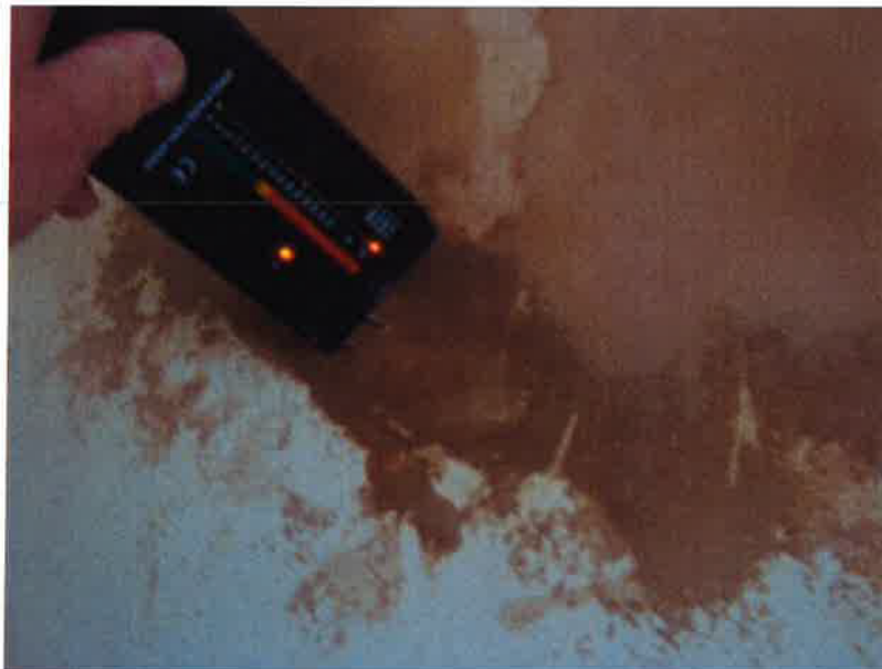
HIGH DAMP READINGS AT CHIMNEYBREAST OF FRONT BEDROOM (17/11/16)
