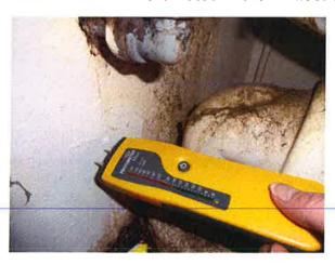
Areas around sink and wc appear to be within normal readings however when removing the bath panel an area of water was noted under the waste pipe showing high moisture readings.
