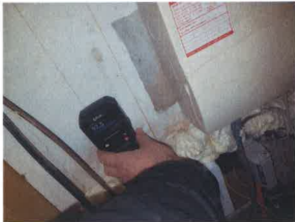
13 High moisture readings within Electrical Cupboard.
