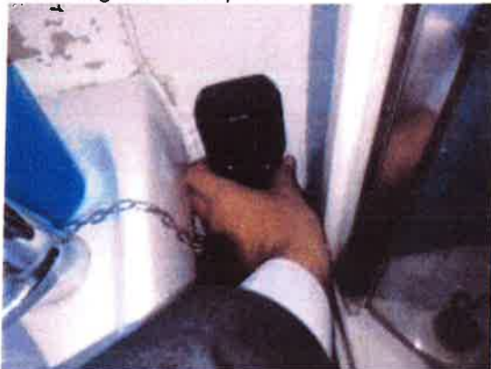
29 High moisture readings adjacent to wash hand basin.
