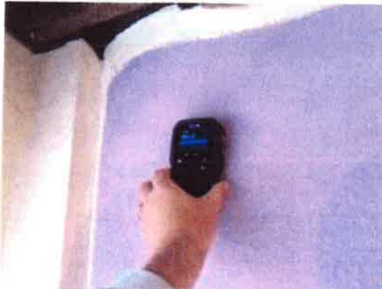
3 High moisture readings within Kitchen at gable wall.
