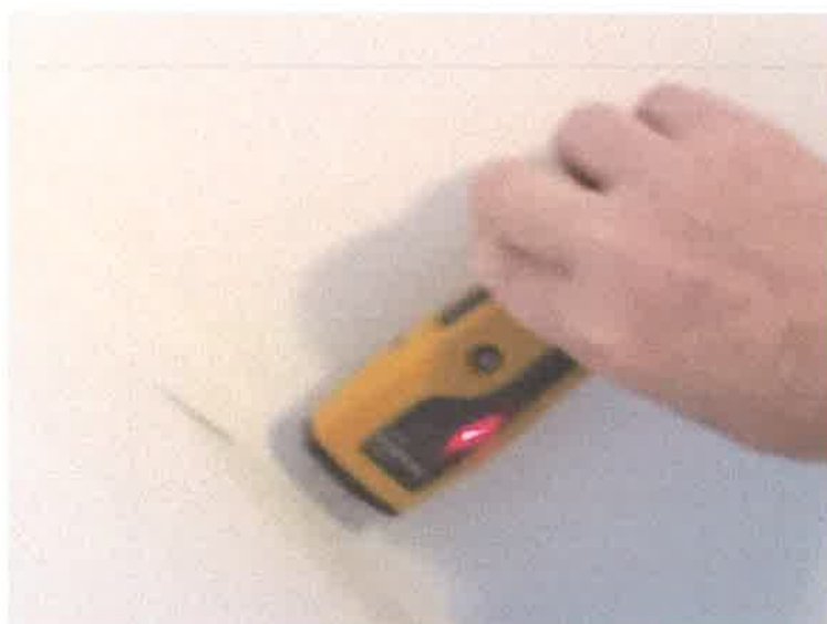
Photograph 13: Bedroom: damp meter reading - junction of ceiling and wall
