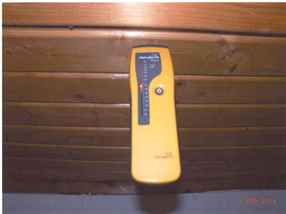
Damp meter reading at Bathroom ceiling
