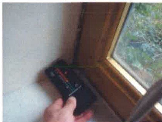
GREEN "DRY" METER READINGS AT LEFT HAND LIVING ROOM WINDOW
