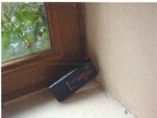
GREEN "DRY" METER READINGS AT LEFT HAND LIVING ROOM WINDOW
