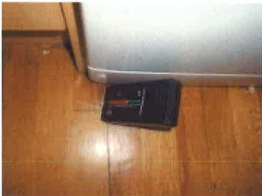
RED “DAMP” METER READINGS AT FLOOR ADJACENT TO WASH MACHINE
