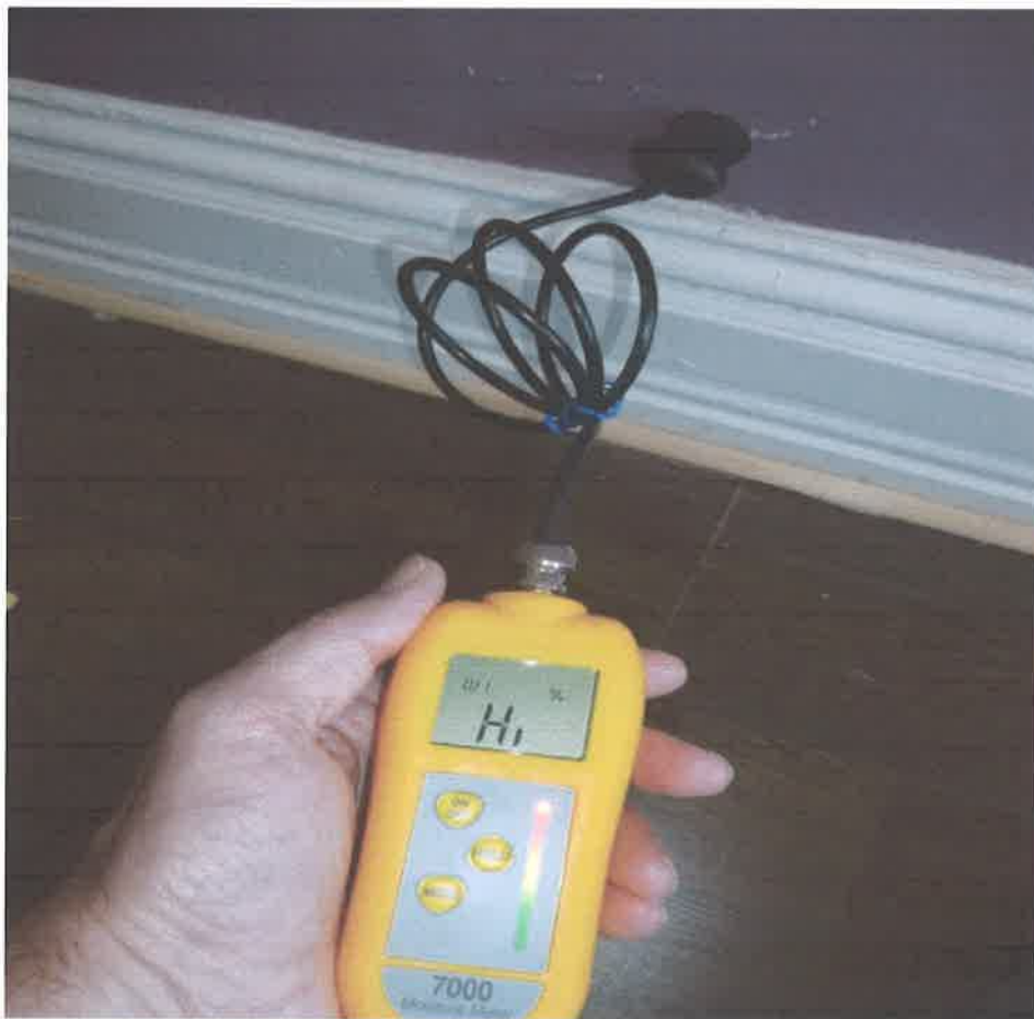
High moisture reading to ex-vent position
