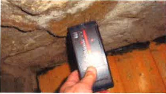
Common Landing – stonework damp.
