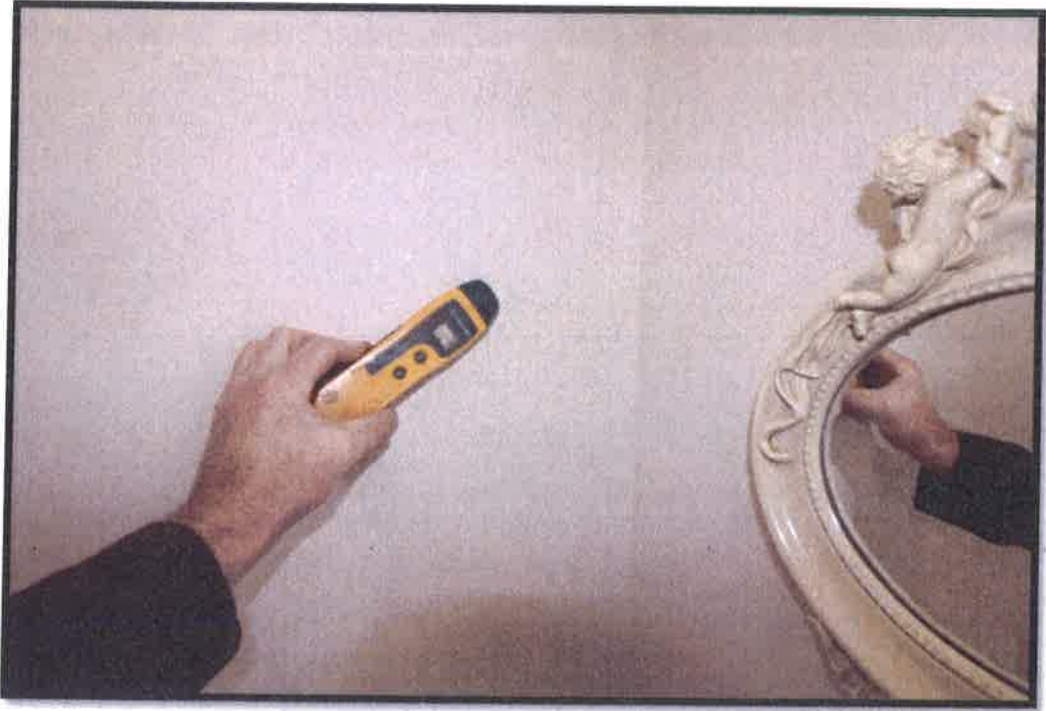
Figure 4 Front Bedroom typical moisture meter reading (11%) (previously 15%)
