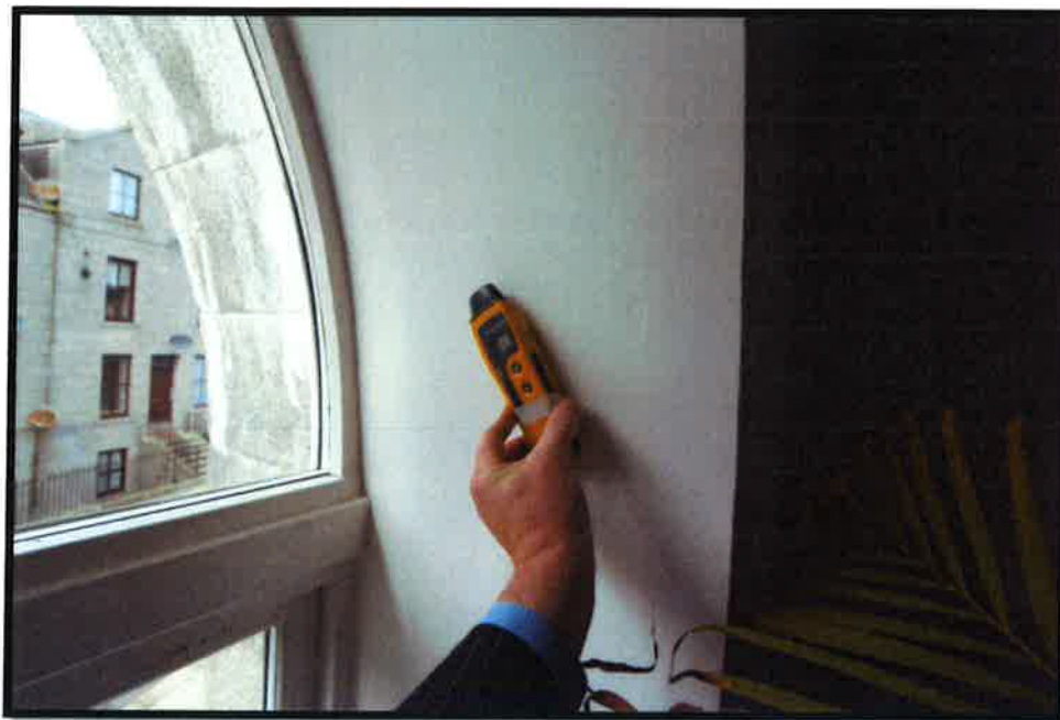
Photograph 6 Meter reading (18%) RHS lounge/kitchen window, mid level.
