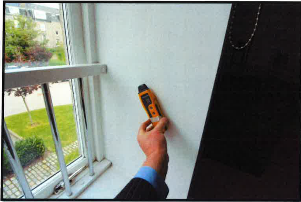
Photograph 10 Meter reading (14%) RHS Master bedroom window.
