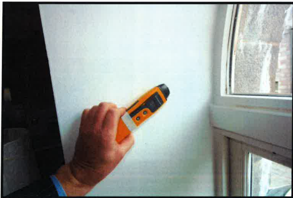
Photograph 5 Further meter reading (20%) LHS lounge/kitchen window, mid level.
