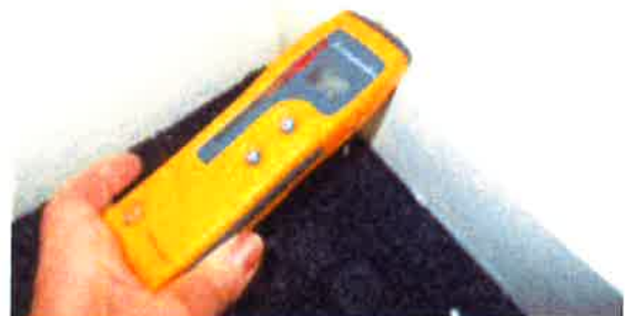
Small Bedroom - high moisture reading to base of external wall to left of window above skirting
