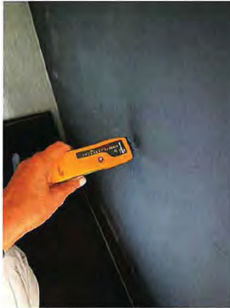
Photograph 15: Bedroom 3: Rear wall – damp meter showing moisture levels in normal range
