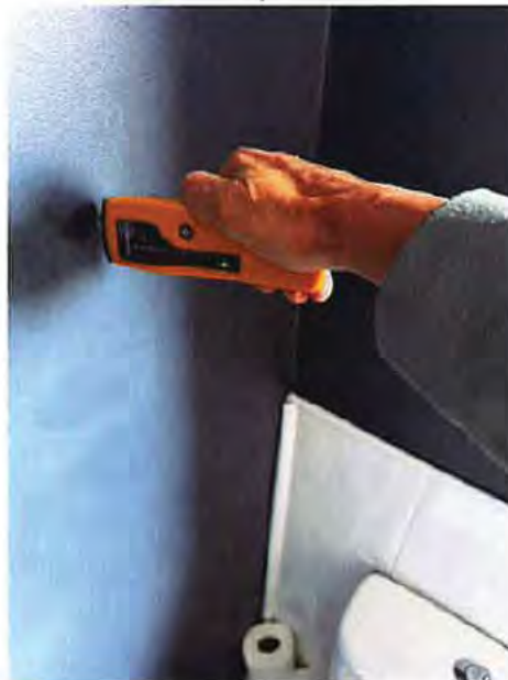
Photograph 19: Bathroom: Side wall - damp meter showing moisture levels in normal range
