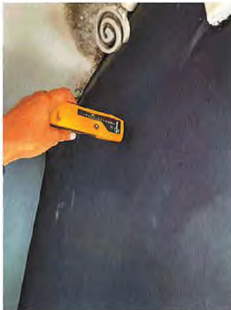
Photograph 15: Bedroom 3: Rear wall – damp meter showing moisture levels in normal range
