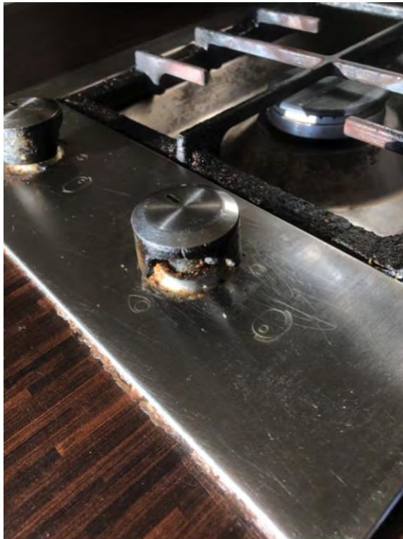
Photo 12 – Broken gas hob dial
