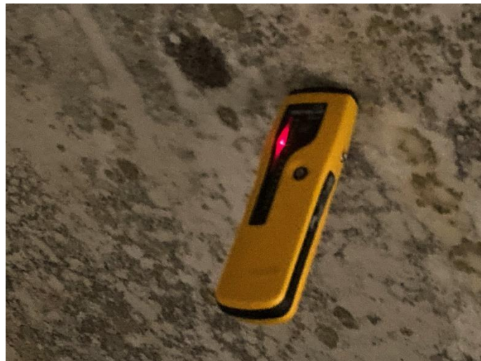
8.Damp "ceiling plaster" in attic
