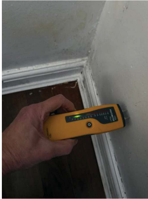
Photograph 3: Bed 1: side internal wall. Normal levels of moisture present.
