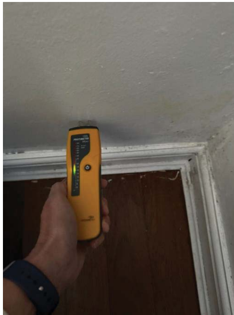
Photograph 3: Bed 1: side internal wall. Normal levels of moisture present.
