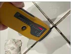
High moisture readings noted around the toilet and along the back wall that has a silicon seal. Grout is missing around some ceramic floor tiles where high moisture readings were also noted.
