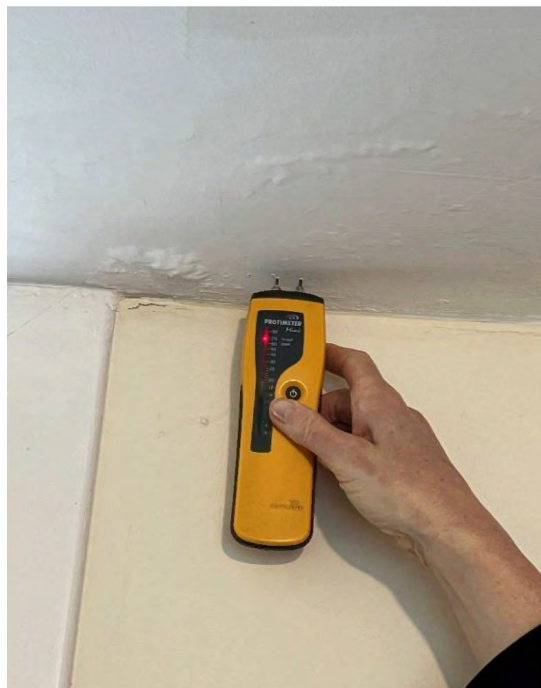
Utility room damp readings present at ceiling 31-07-25
