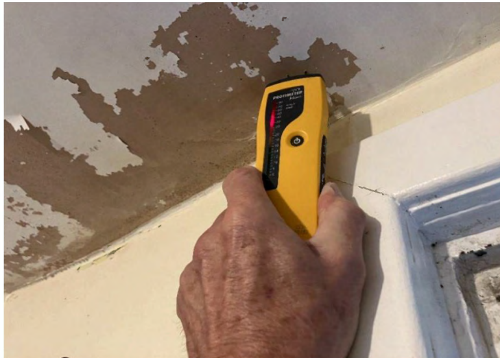
Utility room damp staining at ceiling 14-10-24
