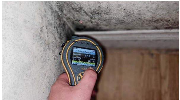
36 Condensation test in Bedroom - surface temperature above dewpoint however surface humidity at 90.7%.
