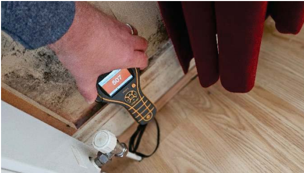
33 Elevated reading at base of wall to Living Room external wall.
