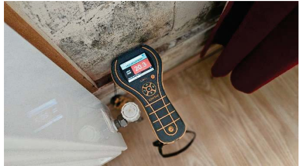
34 Elevated reading at base of wall to Living Room external wall.
