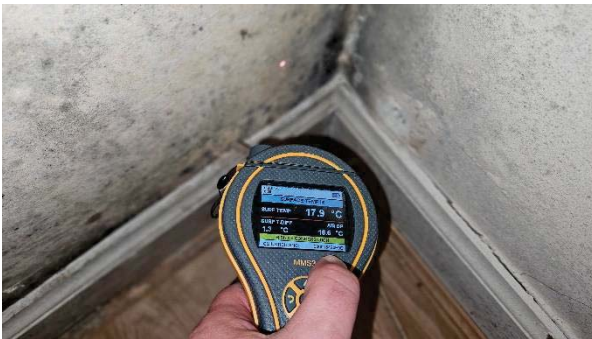
37 Condensation test in Bedroom - surface temperature above dewpoint however surface humidity at 89.0%.
