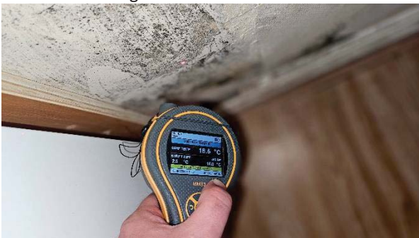
31 Condensation test - surface temperature above dewpoint however surface humidity at 85.7%.
