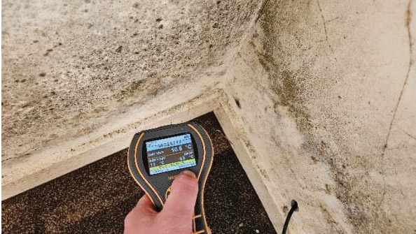
5 Condensation assessment within Eastmost Bedroom, surface temperatures were above dewpoint however, a high surface humidity was recorded.
