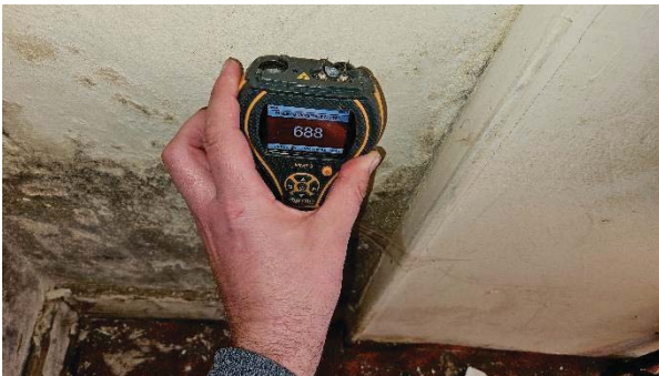
11 Elevated qualitative moisture readings recorded within Hall Cupboard.
