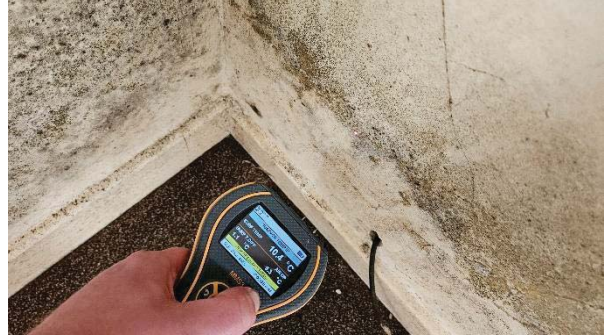
6 Condensation assessment within Eastmost Bedroom, surface temperatures were above dewpoint however, a high surface humidity was recorded.
