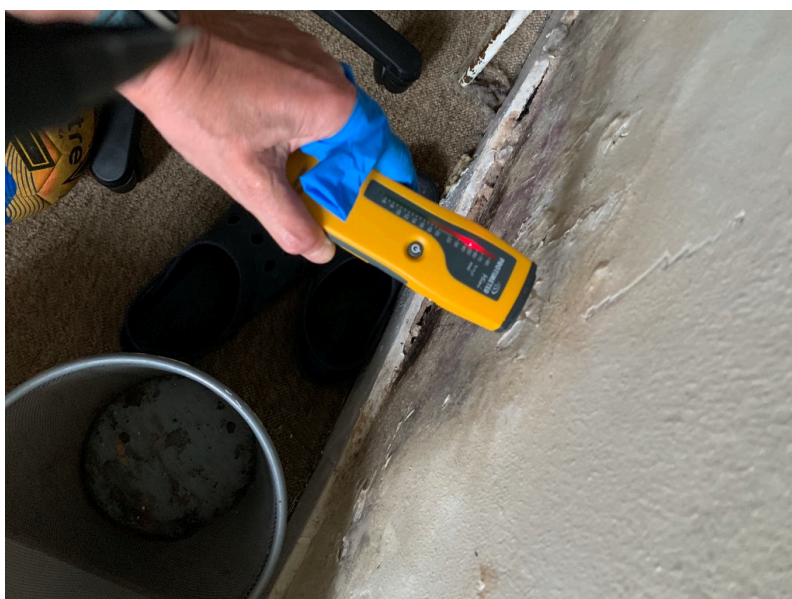
Photograph 19 - showing damp meter readings of high moisture content to left hand internal (adjacent shower room)
