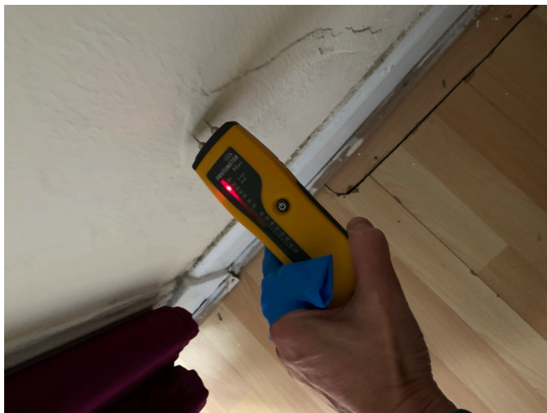
Photograph 5 – showing damp meter readings of high moisture content to rear wall
